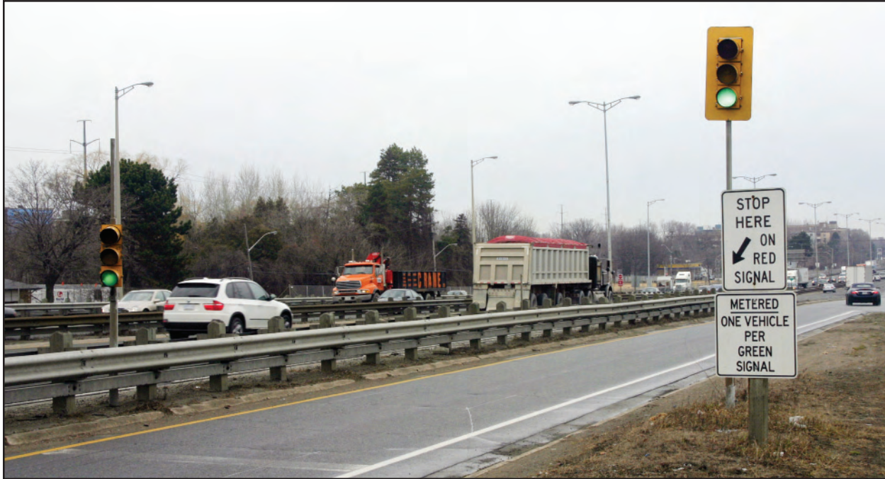
Figure 11 – Signals for Ramp Metering
