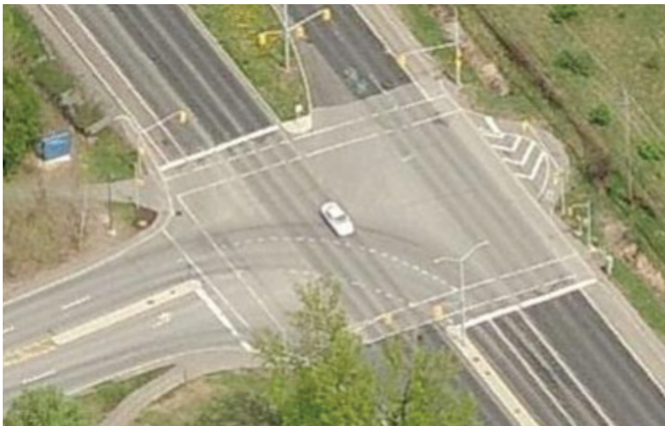
Figure 4.104 – Jug Handle Treatment at Rural T-intersection
