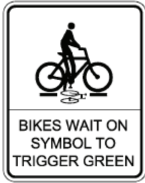
Figure 5.41 – Bicycle Signal Loop Detector Stencil Sign
